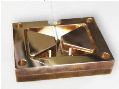
**Fig.1** Photograph of the 3D microwave cavity used in the experiment. The microwave mode of the cavity couples with the ensemble of NV centers in the diamond sample placed inside the cavity.
